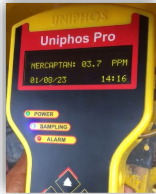
Figure-14: Odourant gas analysis
