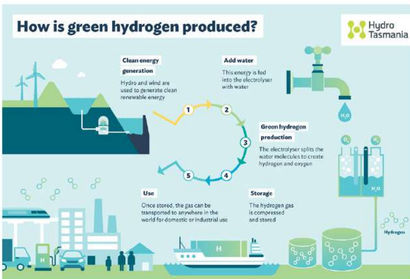
Figure 2 Green Hydrogen Production Process. Source: Hydro Tasmania ( www.hydro.com.au )
